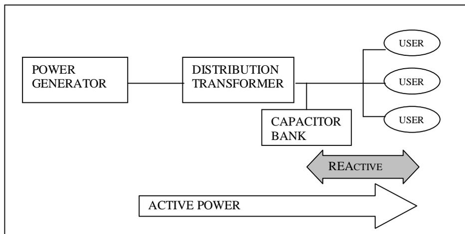
Such system will release the distribution transformer, HT distribution line and the generator of supplying the reactive power, and works out to be a cost effective solution both the user company and the utility company.
